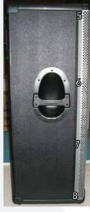
Four screws need to be removed from each side of the grill (eight screws total) using the phillips head screwdriver.
